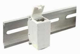
The DIN rail coupler is in compact design for mounting on DIN rail TH35 according to DIN EN60715. The Cat.6A/Class EA screened coupler supports the 10G cabling and is 4PPoE compliant. Plastic casing with capability of grounding to the DIN rail is most ideal device for application in accordance with rule VDE-AR-N 4100: 2019-04. The coupler is IP20, supplied with dust covers and can be mounted side by side.
